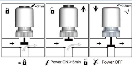
N/C normally closed(First installtion of power on/off indication )
