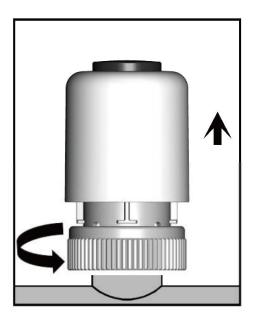
Rotate the nut anticlockwise until remove the actuator ( (Note: Do not use pipe pliers, clamp and other tools)
