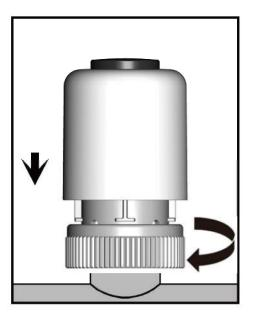
Rotate the nut clockwise and install it on the valve (Note: Do not use pipe pliers, clamp and other tools)
